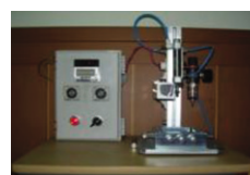
• Fig 2. The device which is designed for the fatigue test
